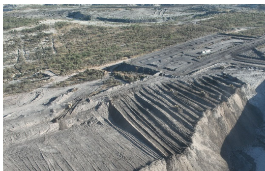
Bulk dozer push operations at Blair Athol for coal exposure
